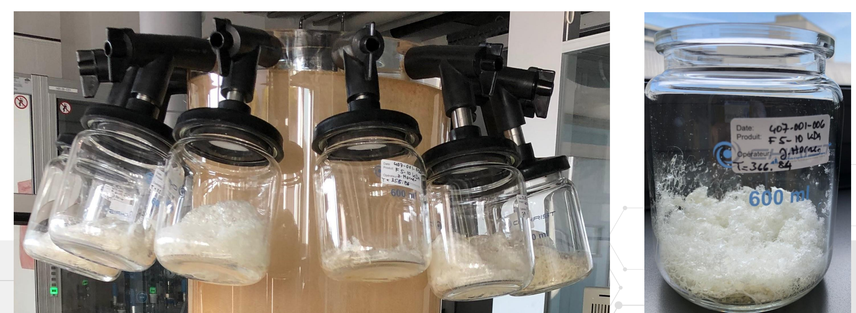
Freeze-drying of the different peptide fractions of the scaled-up hydrolysates to gently remove water and obtain stable peptide format
